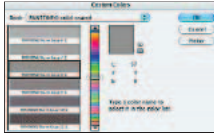
FIGURE 5-28. CUSTOM COLORS. Access the Color Picker or Custom Colors options by clicking on the ink color square in the Duotone Options dialog box.
